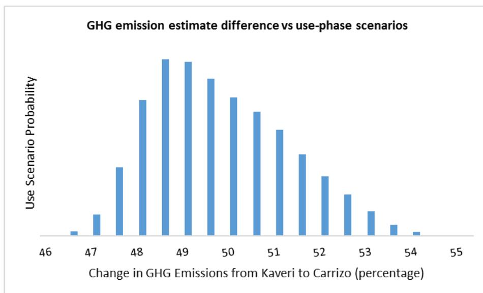
Figure 5: Use phase scenario probability vs GHG emissions estimate difference (%) with variations in off, sleep, long and short idle modes for a simulation of 10,000 random use cases<sup>xxvi</sup>
