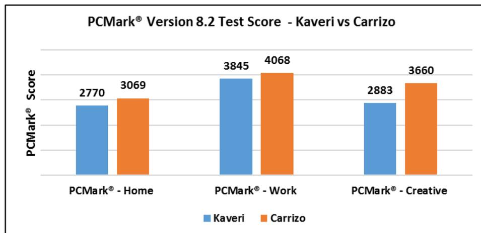
Figure 2: Test results from AMD Power and Performance Lab on PCMark® Version 8.2<sup>xi</sup>
