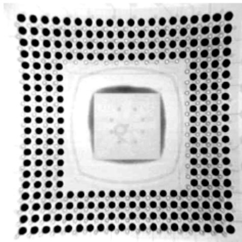
X ray image of PBGA unit, shows alignment Ball to pad.
