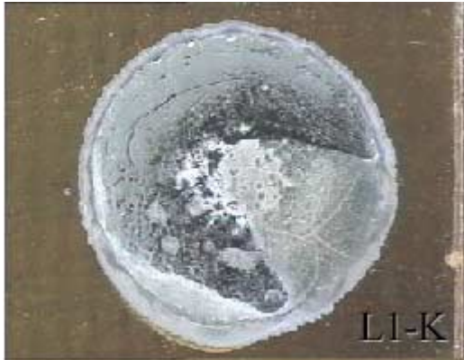
Paste: Kester; Profile Linear
