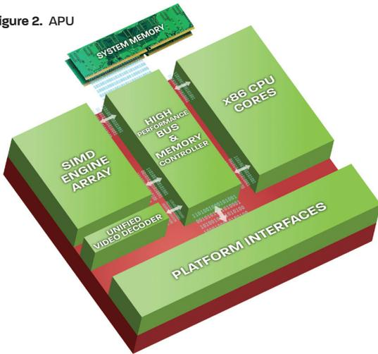
Until now, transistor budget constraints typically mandated a two chip solution for such systems, forcing system architects to use a chip-to-chip crossing between the memory controller and either the CPU or GPU as shown in Figure 3. These transfers affect memory latency, consume system power and thus impact battery life. The APU's scalar x86 cores and SIMD engines share a common path to system memory to help avoid these constraints.
