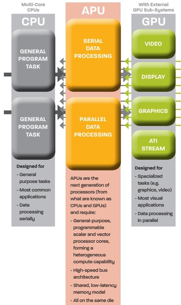
Figure 2 illustrates the arrangement of these first APUs. The key aspect to note is that all the major system elements – x86 cores, vector (SIMD) engines, and a Unified Video Decoder (UVD) for HD decoding tasks – attach directly to the same high speed bus, and thus to the main system memory. This design concept eliminates one of the fundamental constraints that limits the performance of traditional integrated graphics controllers (IGPs).
