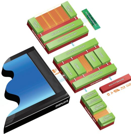
Total system performance can be further enhanced through the addition of a discrete GPU. The common architectures of the APU and GPU allow for a multi-GPU configuration where the system can scale to harness all available resources for exceptional graphics and enable truly breathtaking overall performance.
