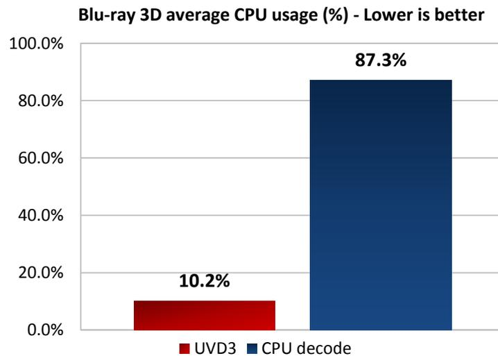
**Figure 4: Example of CPU utilization during Blu-ray 3D<sup>3</sup> playback**
