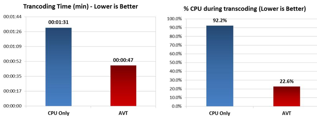
**Figure 9: AVT transcoding speed and CPU usage**
