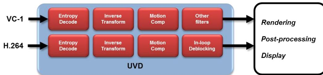
Figure 1: 1<sup>st</sup> generation Unified Video Decoder
