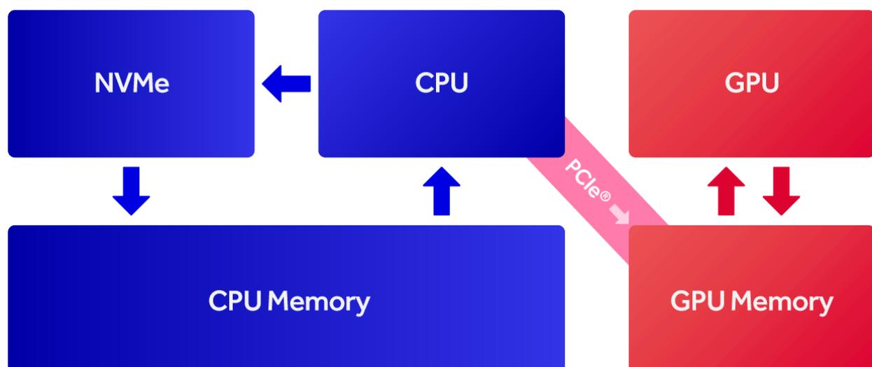
Figure 2: Data path for typical graphics transaction necessitates many copy transactions that are expensive to process.
