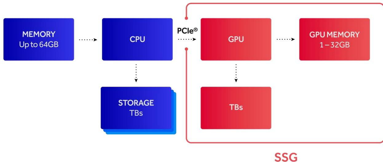
*Figure 3: The system storage architecture with Radeon™ Pro SSG.*
