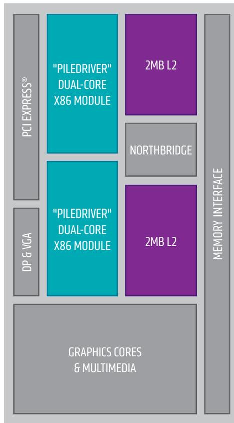
*Integration of large GPU cores, as done in AMD R-Series APUs, increases the potential for unused power budget.*
