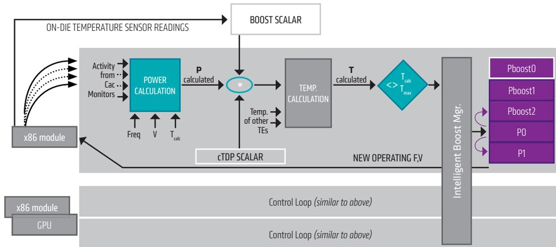
AMD Turbo CORE algorithms use a variety of frequency, voltage, temperature and logic activity inputs to dynamically determine which cores need a performance boost and how much thermal headroom is available.
