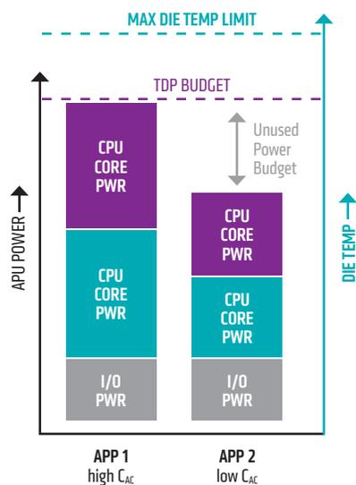
*Applications with a low  $C_{AC}$  can leave unused TDP and temperature headroom. New power management techniques can exploit both for improved performance.*
