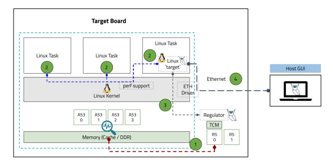
Architect is composed of software components running on the "target board" (e.g., Kria KV260 Starter Kit) and by the graphical user interface (GUI) running on the developer/integrator Host PC.
