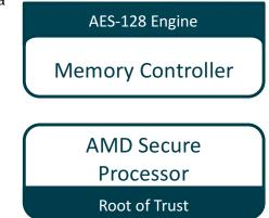
AMD EPYC processors combine these components to offer two new security features:
