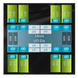
Figure 3 Single socket EPYC 7002 Processor internal connection between CCDs and Memory through the IOD via Infinity Fabric
