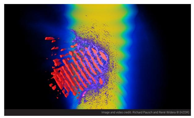
PIConGPU simulation of a cryogenic hydrogen jet interacting with a high-intensity laser beam, a model of an experiment recently performed at Helmholtz-Zentrum Dresden-Rossendorf (HZDR) at the DRACO laser system.
