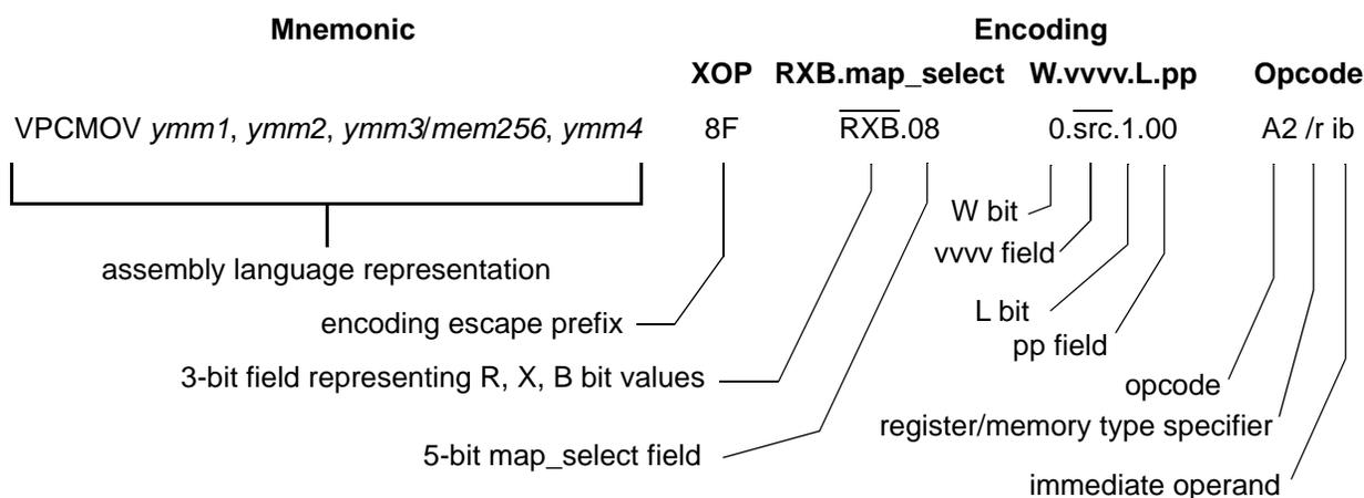
**Figure 1-1. Typical Descriptive Synopsis - Extended SSE Instructions**
