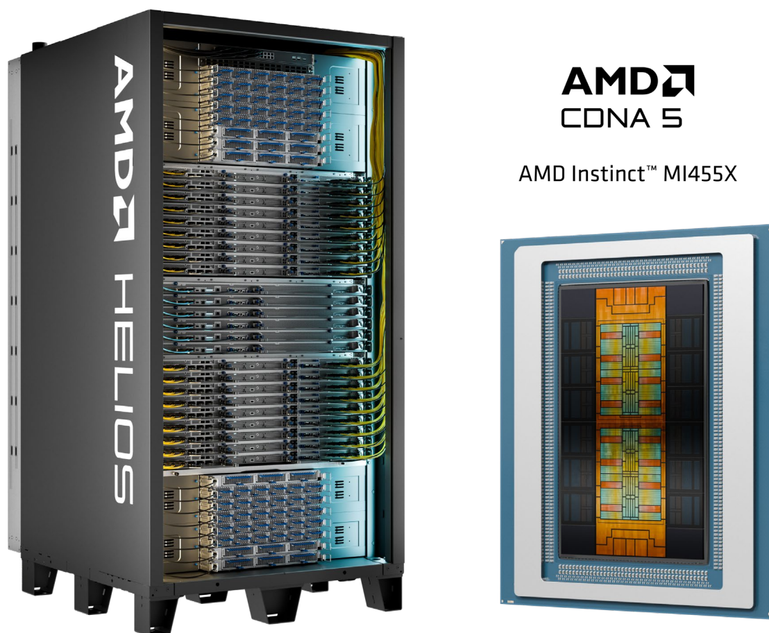
Figure 1. The AMD Helios™ rackscale solution and the AMD Instinct™ MI455X GPU.
