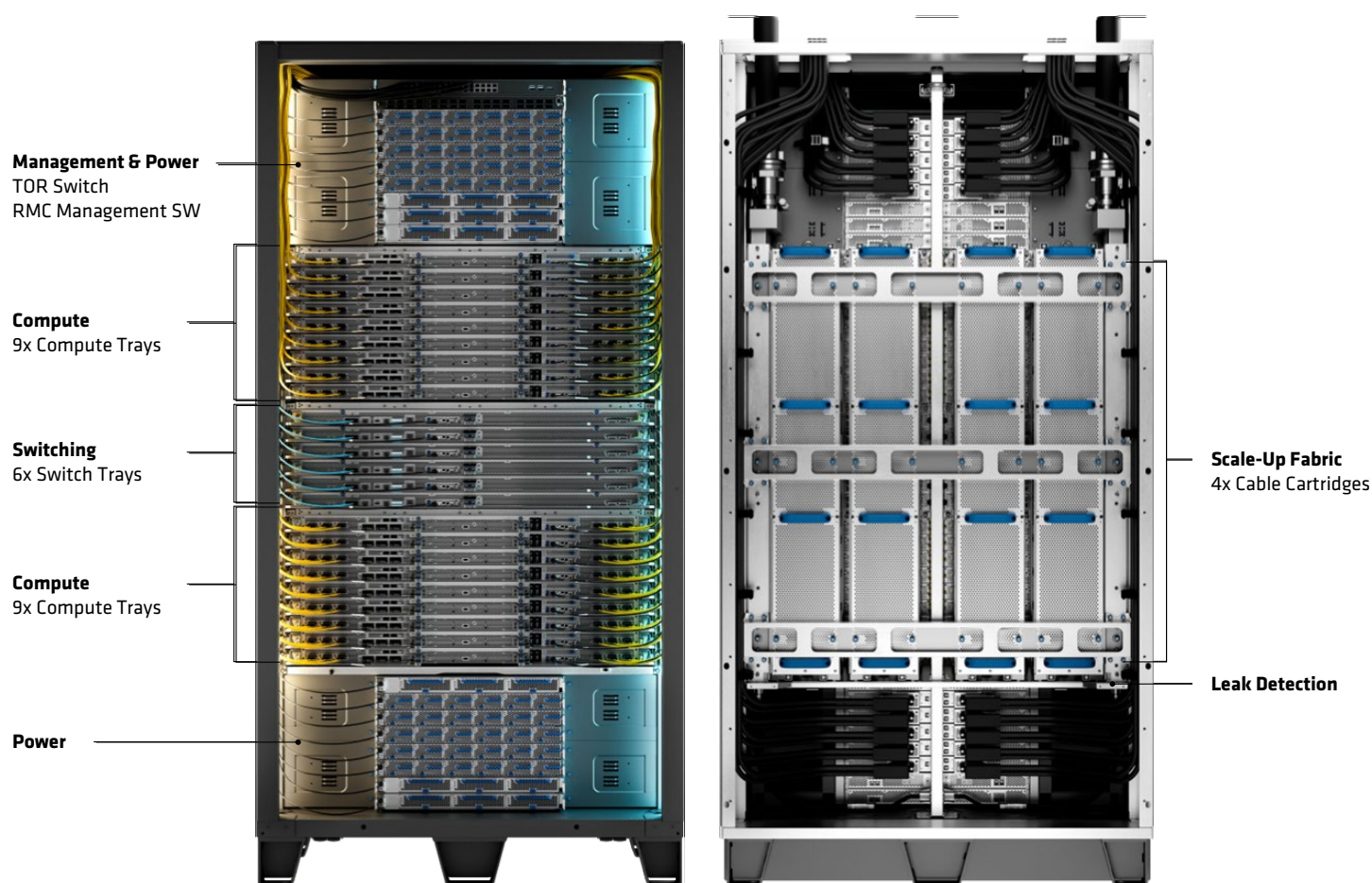
Figure 9. Front and rear view of the AMD Helios™ rackscale solution.
