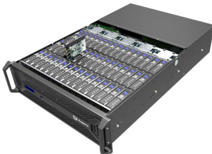
Figure 1: The Aup2600 features 48 AMD Zynq MPSoC devices
