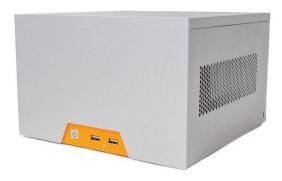
The MC850-40 incorporates an AMD Ryzen<sup>™</sup> 3rd Generation 3950X processor, includes 4 USB ports, 2 10Gb LAN ports, 1 IPMI, and offers up to 64 GB DDR4 SO-DIMM memory and dual 2.5" SATA storage drives. It provides extremely fast storage and capable connectivity in a small device.
