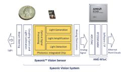
Both application spaces have been widely demonstrated by SiLC. Furthermore, the processing backbone of the Zynq UltraScale+ RFSoC allows for implementation of advanced LiDAR processing algorithms running in real time on this 40 GSPS aggregate data rate coming from the 8 ADC channels. The flexibility of the RFSoC fabric allows for frequent algorithm updates and has played a pivotal role in SiLC's innovation roadmap over the past few years.
