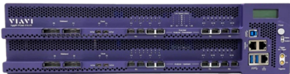
Figure 1: Image of Xgig 6P16 analyzer/exerciser for PCI Express 6.0
