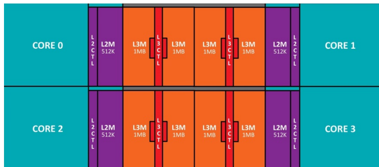
EPYC's CPU Core Complex (CCX) Four Cores and 8MB L3 Cache
